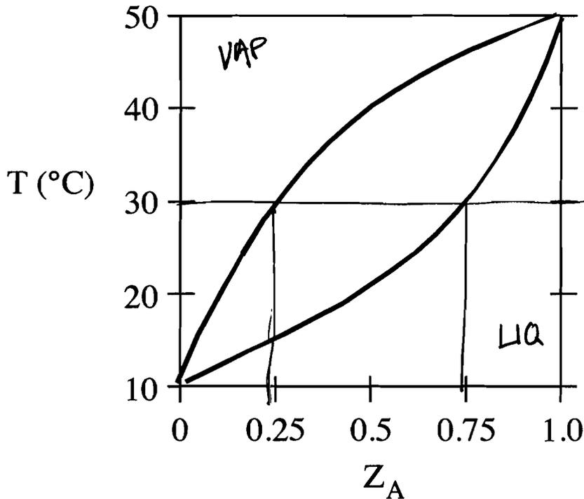
The temperature composition diagram for binary mixture of two compounds A & B at a pressure of 1 bar is given above. Assume the vapors are ideal gases and the mixture is an ideal mixture.
