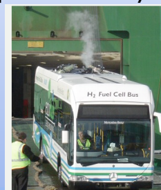
In the photograph above the fuel bus is unloaded from the ship, with the pure steam rising from its exhaust pipe visible at the rear.
