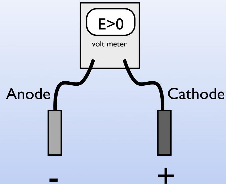
Cathode at a higher potential than the anode
