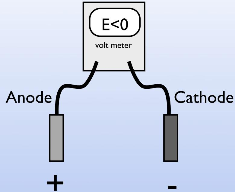
Anode at a higher potential than the cathode
