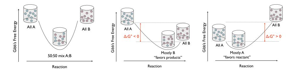
The case where  $\Delta_r G^\circ = 0$  is on the left. The lowest free energy state is the state with equal number of molecules of A & B. This is the state with the highest entropy. Neither pure state has any entropy from mixing. Thus the even though A and B have identical free energies, the lowest free energy is in the 50/50 mixture. Higher entropy leads to lower free energy (G = H –TS). So the equilibrium mixture will be right in the middle.
