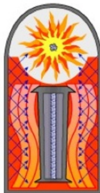
4. Polystyrene foam becomes plasma, compressing secondary, and plutonium sparkplug begins to fission.
