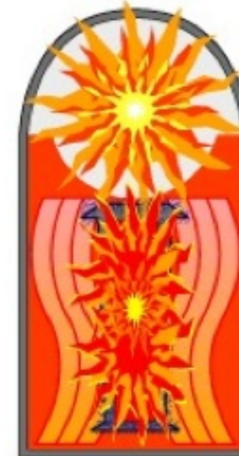
5. Compressed and heated, lithium-6 deuteride fuel begins fusion reaction, neutron flux causes tamper to fission. A fireball is starting to form...
