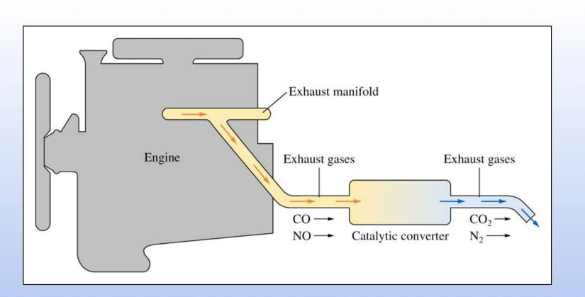
Catalyzes three chemical reactions  $2NO_x \longrightarrow xO_2 + N_2$   $2CO + O_2 \longrightarrow 2CO_2$  $2C_xH_y + (2x+y/2)O_2 \longrightarrow 2xCO_2 + yH_2O$
