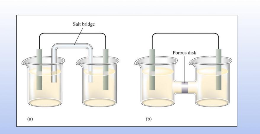
Salt Bridge or Porous Disk allow ions to flow back and forth between the two beakers. As e<sup>-</sup> move from one side to the other, counter anions move the opposite direction
