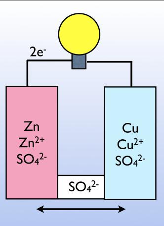
Add a connection that let's a "counter" ion move between the two sides
